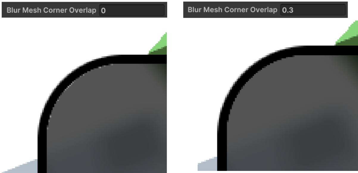
The corner OVERLAP defines how much further out the blurred mesh should be drawn in order to cover up these gaps. Usually a value of about 0.2 or 0.3 is fine.
