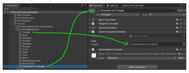
**NOTICE:** The forwarder uses the rect shape of the hole to make an area clickable. The "Target" mustn't be a hold object. It can be any transform its area you want to enable click-through. The forder has to be IN FRONT (meaning at the lowest position in the hierarchy) within the mask to work.
