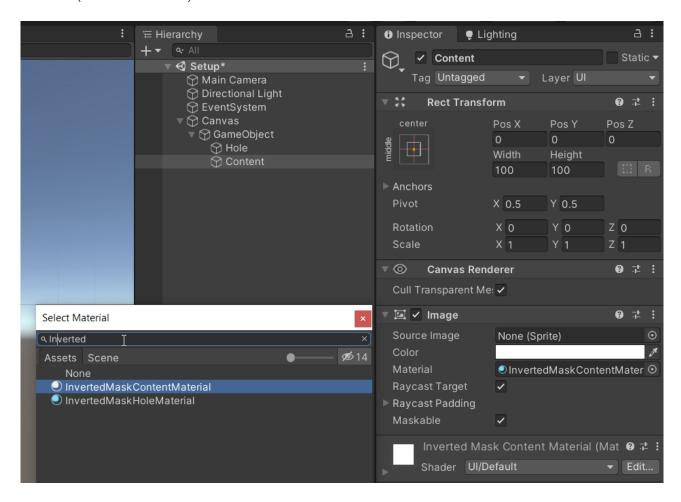
Second we need to add the **InvertedMaskHoleMaterial** to the **Hole** Image.
