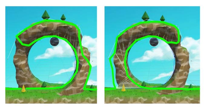
Now the remaining problem is the position of the object in depth. The object (the ball) has to move back to avoid a visual collision with the terrain (notice the difference between ball *z* position and the 2d collider position).
